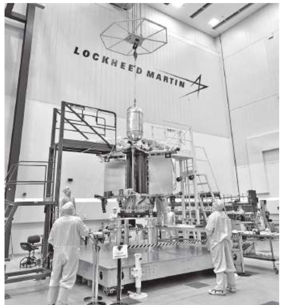
Engineers install Lucy's oxygen propellant tank into the spacecraft structure in a high-bay clean room at Lockheed Martin.
