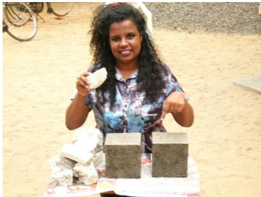
The Author displaying the concrete blocks made from Tsunami debris
