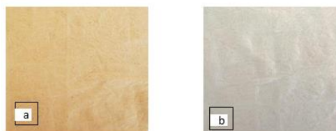
Figure 2.24 samples pre mordanted with ferrous sulphate (a) and copper sulphate (b)
