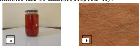
Figure 2.14 Thespesia populnea extracted dye at 100°C over 30 mins (a) with dyed sample (b)
