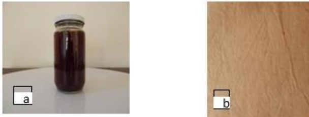
Figure 2.2 Thespesia populnea extracted dye at pH 5 (a) with dyed sample (b)
