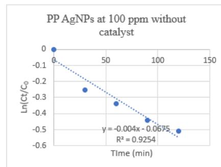
Figure 28: Photocatalytic kinetic graph of PP AgNPs at 100 ppm without catalyst
