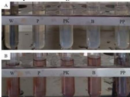
Figure 7: Biosynthesis of AgNPs using Petunia leaf extracts. The AgNO<sub>3</sub> solution changed from pale yellow (A) to deep brown (B).
